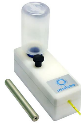
Manual ball sealer for 0.5 ml straws
