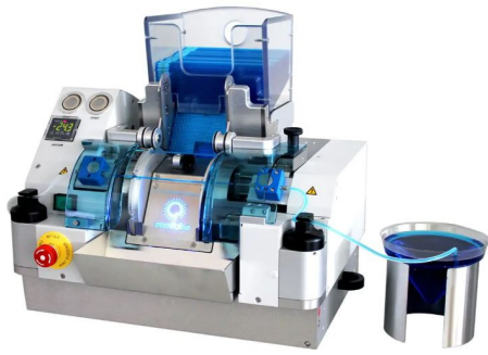
MPP Uno, automatic filling and sealing machine for semen straws
